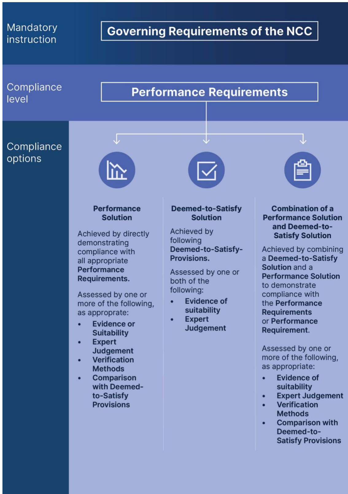
Figure C. 1 Demonstrating compliance with the NCC
